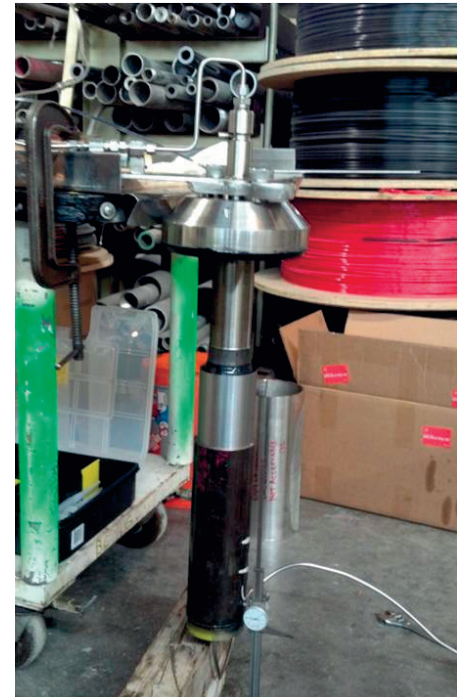
Figure 5 Packer Final Construction
