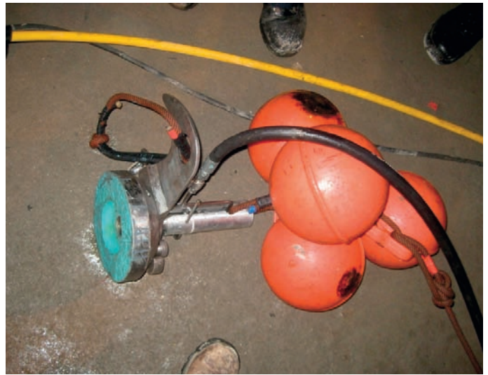
Figure 8 Packer Cap with Floats for Retrieval after Disconnect
