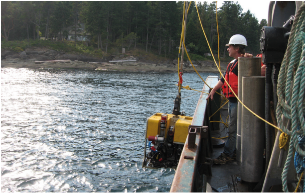
Mohican ROV live boat configuration for cable lay and bottom surveys.
