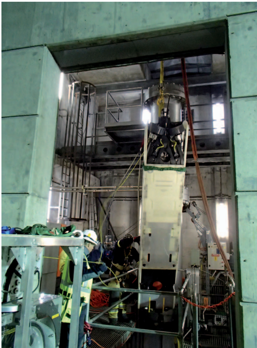
Hibbard Inshore Saab long tunnel inspection vehicle entering tunnel through narrow shaft.
